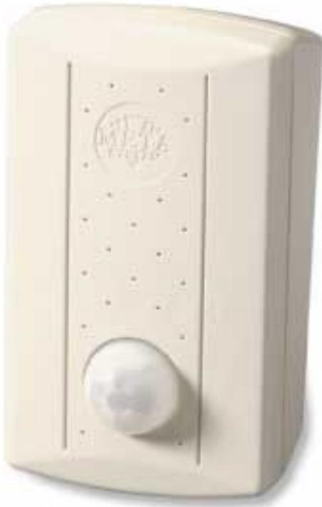
Dual-technology wire-less device for domestic protection using a passive infrared sensor (able to detect the heat of the human body in movement) combined with a microwave movement detector.
